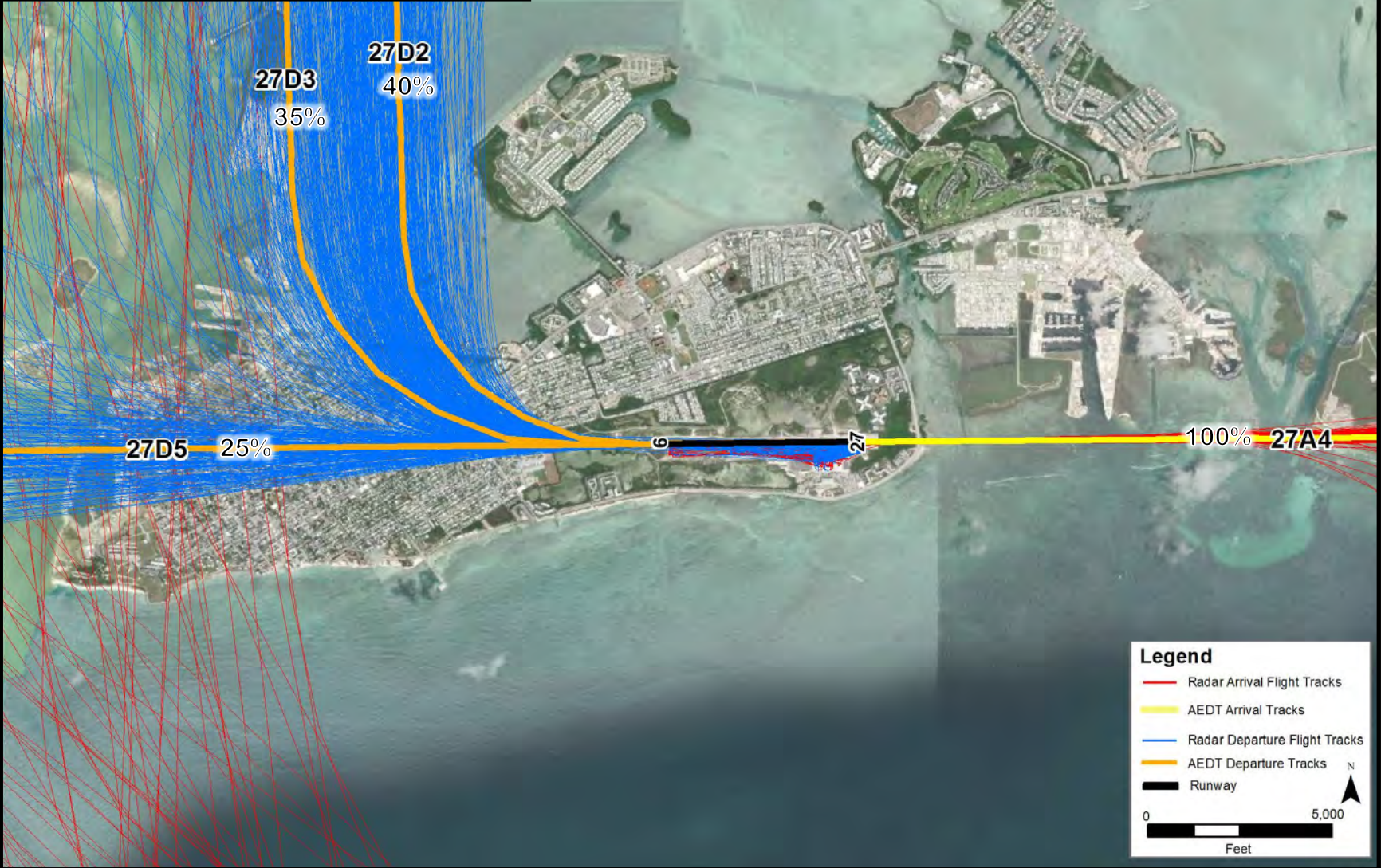
WEST FLOW AC/AT JET FR24 FLIGHT TRAJECTORIES WITH AEDT MODELED FLIGHT TRACKS AND UTILIZATION
