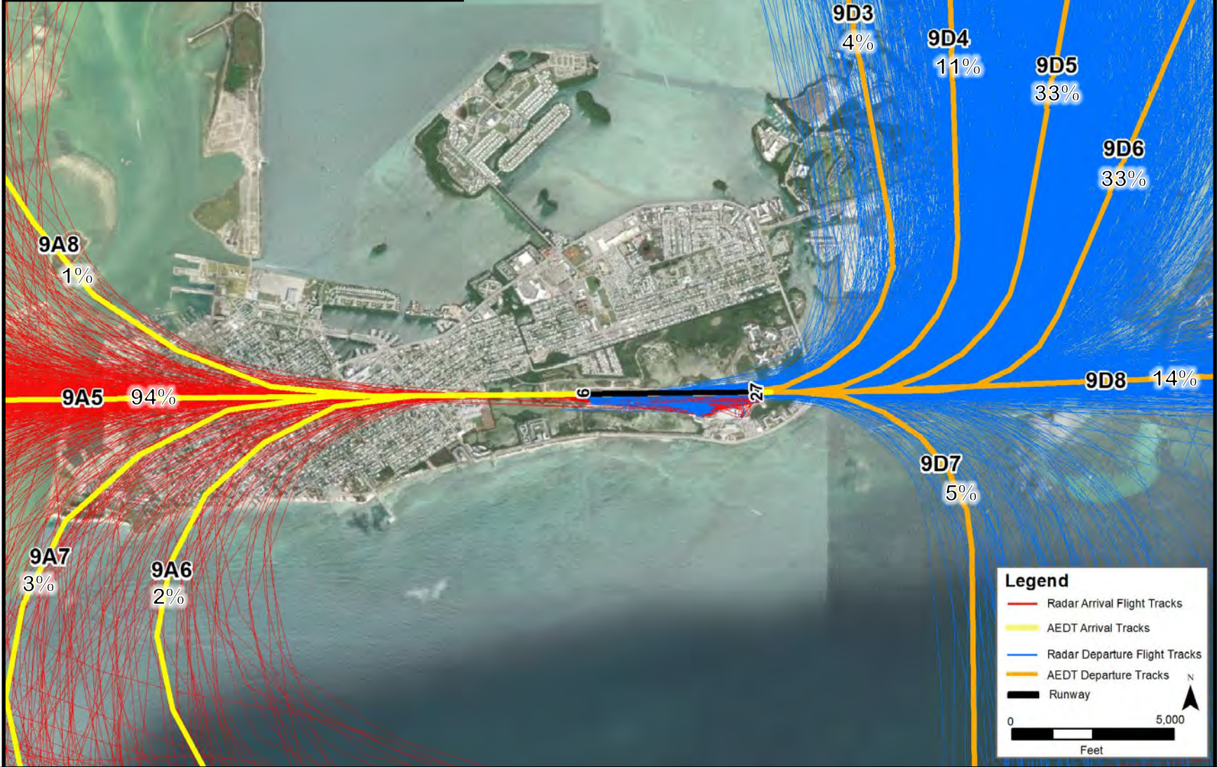
EAST FLOW GA JET FR24 FLIGHT TRAJECTORIES WITH AEDT MODELED FLIGHT TRACKS AND UTILIZATION
