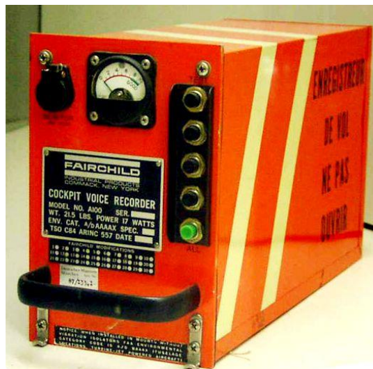
Figure 2. Representative Cockpit Voice Recorder
